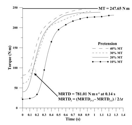
Fig. 3 Graphical illustration and the equation for calculating the slope of the torque time curve (*MT* maximum torque; *MRTD* maximum rate of torque development)
